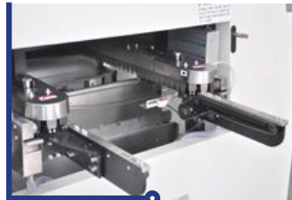
Titanium finger conveyor includes motorized width adjustment and PC software control
