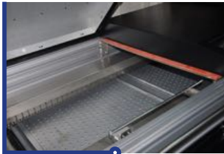
Hot air preheating zone with 1800mm length
